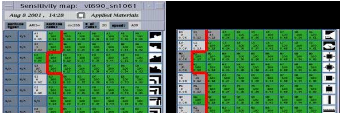
Figure 1: Comparison of AAPSM and standard A09 inspection sensitivity using the VT690 mask. The red line represents the standard ARIS100i sensitivity for binary masks (100% capture rate). The PSM sensitivity is very compatible for almost all defect types. Only for truncation defects (VT types I and K) the A09 is slightly better than the AAPSM.
