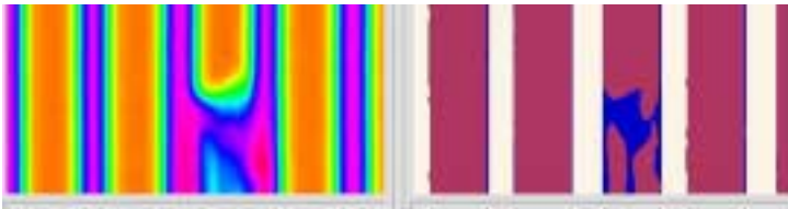
Figure 10c: Inspection image of missing chrome defect (left) and overlay with database (right). The reason of this defect could be a defective mask blank.
